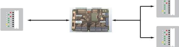
Use two Communication Modules to link up to eight Annunciators via RS485, LAN/WAN or a wireless transmitter
