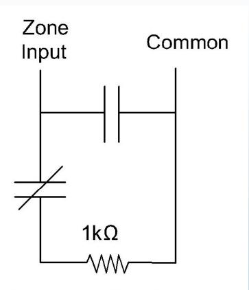
Normally Closed and Normally Open Contact with EOL resistor
