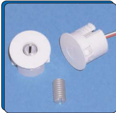
MAGNET HOLDER AND \varnothing 1/4" \times 1/2" RARE EARTH MAGNET MAGNET HOLDER SCREWS IN AND OUT TO ADJUST GAP
