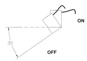
The **Flair Tilt Switch**, **P/N TSS235**, is a rugged security device for protecting many objects from being moved or tampered. With the case vertical and wires up, as shown above, the circuit is closed. Tilting the switch in any direction more than 35 Degrees will open the circuit. Use tape provided to mount Switch to any vertical or horizantal surface
