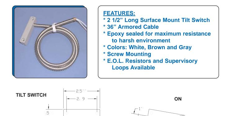
The **Flair Tilt Switch**, **P/N TSS5310**, is a rugged security device for protecting many objects from being moved or tampered. With the switch horizontal, as shown above, tilting the switch up around the wires will close the circuit. Tilting the switch down will open the circuit. Switch may be mounted bottom or side with screws or tape.
